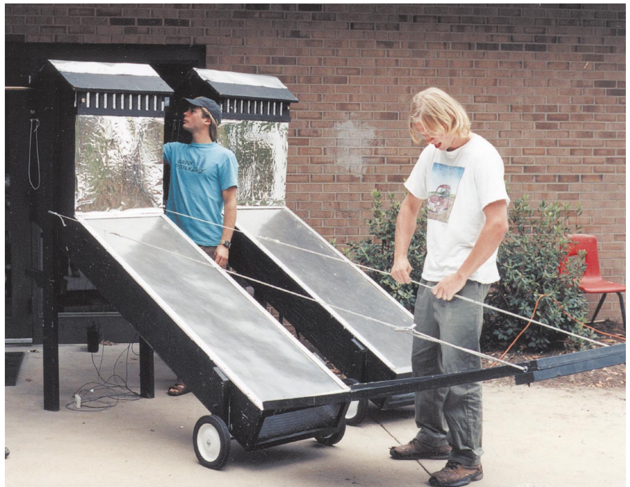
Above, Photo 4: Setting the front reflector angle.
